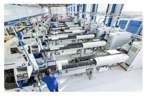
What does this profession involve? Bar turning is a cutting-edge sector in which France is a world leader. As a precision mechanic, the bar turner manufactures small parts in series from bars mounted on machines called bar turning lathes, either automated or numerically controlled.
